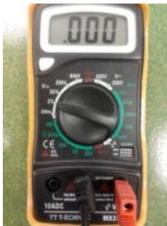
Figure 3(a): Voltmeter Setting
