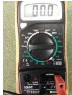
Figure 3(b): Ammeter Setting
