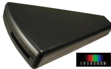
Figure 1: Hand held spectroscope qualitatively determines the wavelength of light.
